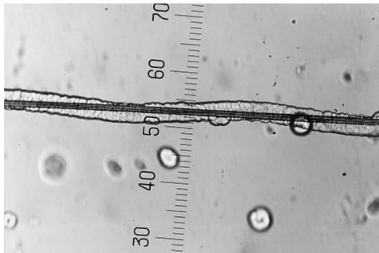
Fig. 19. A photograph of \alpha transcrystalline layer grown on Kevlar 149 fibre, showing the typical helical formation.
